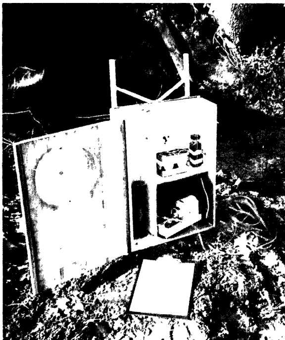
Figure 11.—Backpack dye-injection apparatus in use.
