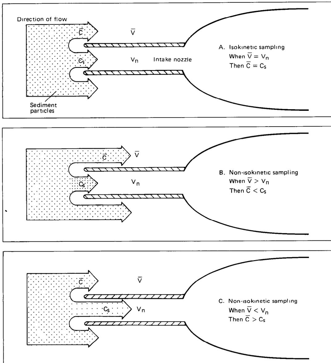
**Figure 11.** Relation between intake velocity and sample concentration for (A) isokinetic and (B, C) non-isokinetic sample collection of particles greater than 0.062 mm. When  $\bar{V}$  = mean stream velocity,  $V_n$  = velocity in the sampler nozzle,  $\bar{C}$  = mean sediment concentration in the stream, and  $C_s$  = sample sediment concentration.
