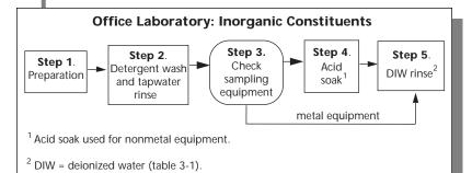
Figure 3-2. Office-laboratory cleaning procedures for equipment used to sample for inorganic constituents.
