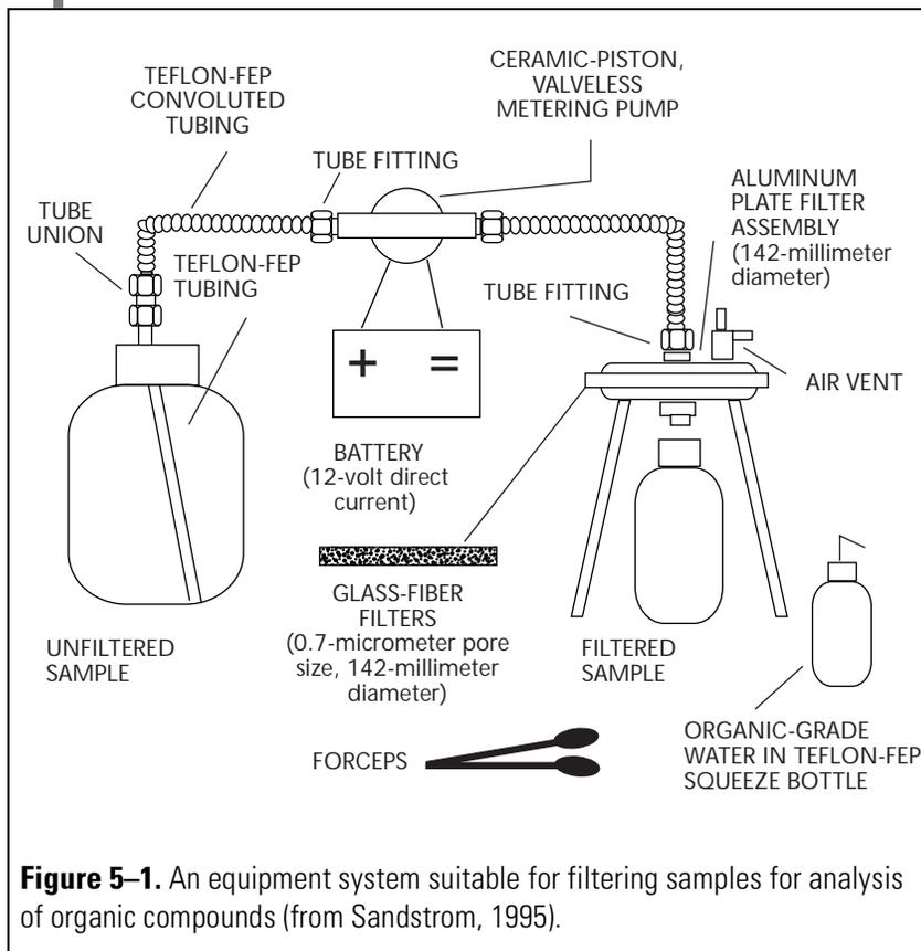
**Figure 5-1.** An equipment system suitable for filtering samples for analysis of organic compounds (from Sandstrom, 1995).
