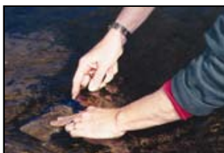
f. A soft substrate, epipellic sample being collected with the inverted petri dish method. Note how a spatula is placed beneath the petri dish to keep the sample intact.
