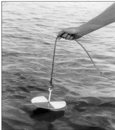
Figure 7.4–3. Lowering a Secchi disk into water. (Photo provided by Kent State University, Ohio.)
