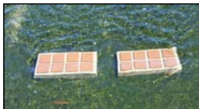
e. Example of an artificial substrate sampler using clay tiles placed on concrete pavers.
