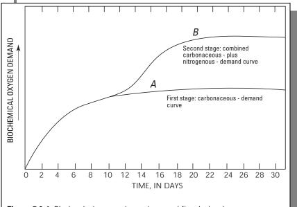
**Figure 7.0-1.** Biochemical oxygen demand curves: (*A*) typical carbonaceousdemand curve showing the oxidation of organic matter, and (*B*) typical carbonaceous- plus nitrogeneous-demand curve showing the oxidation of ammonia and nitrite. (Modified from Sawyer and McCarty, 1978.)
