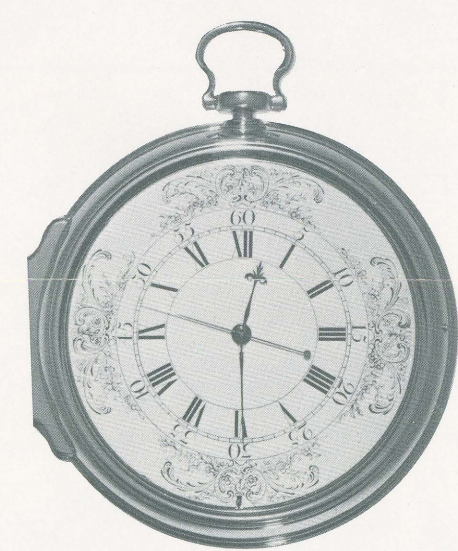
ca. 1761—John Harrison's marine chronometer number four. This was the earliest accurate way of measuring longitude at sea.
