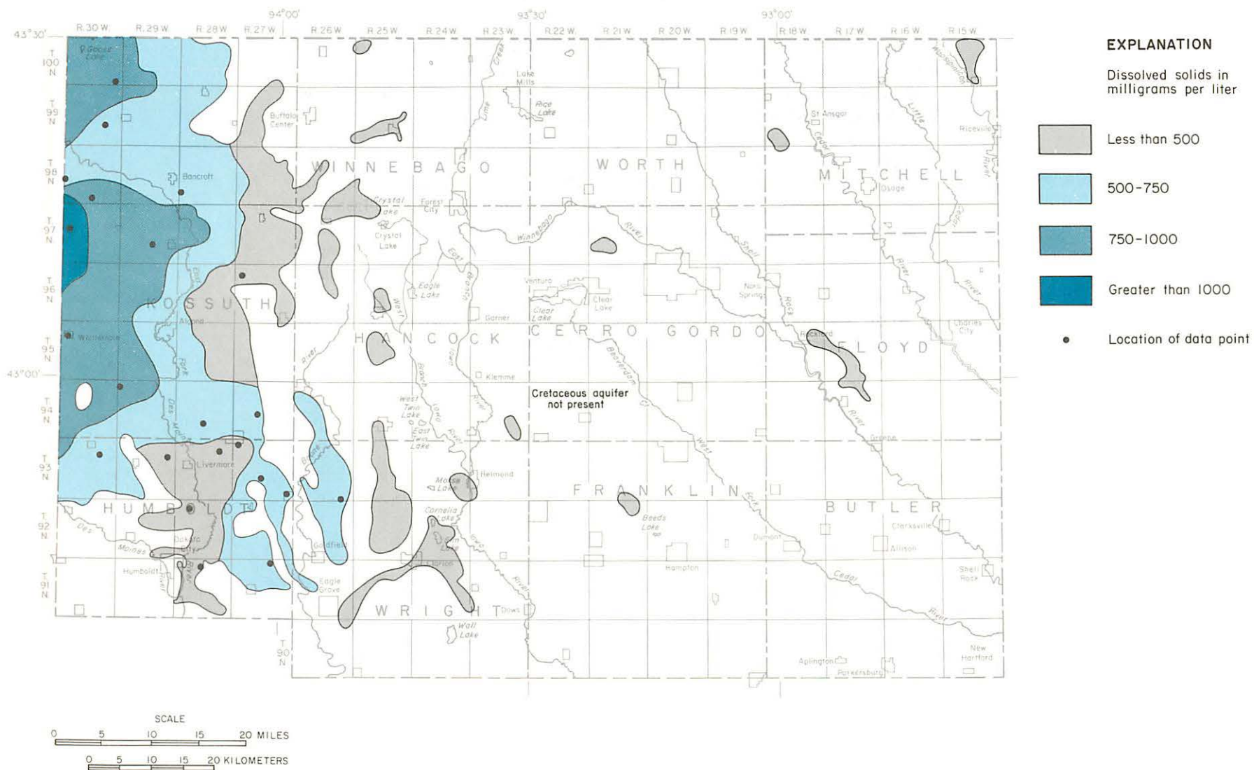
Figure 56. Dissolved-solids concentration in water from the Cretaceous aquifer
