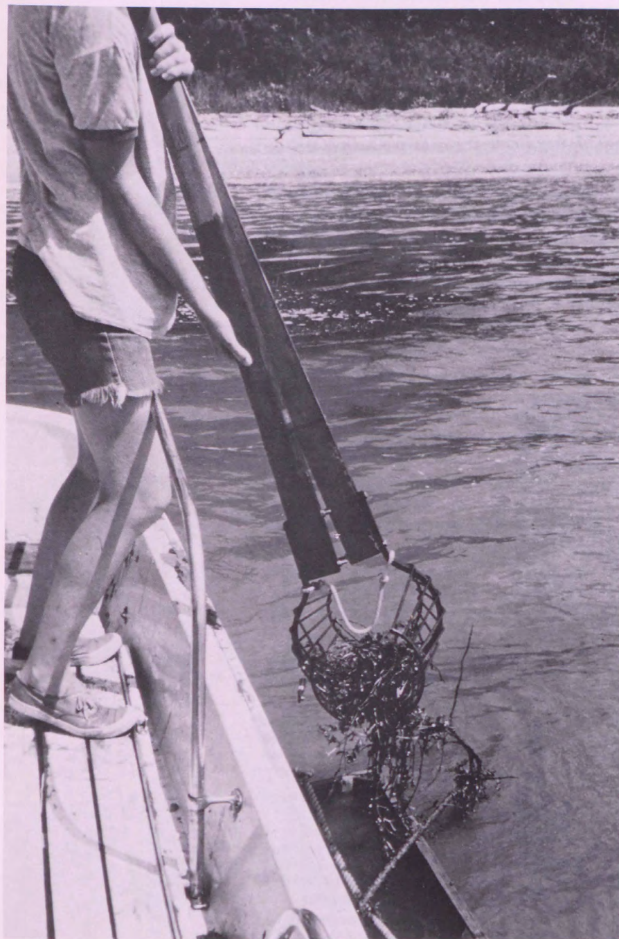
Sampling submersed aquatic vegetation and substrate with modified oyster tongs.
