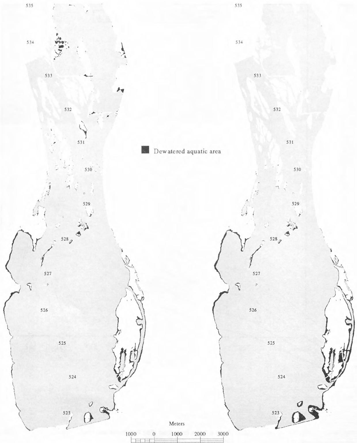
Figure 7. Maps of Pool 13 depicting areas dewatered from a 1-foot drawdown at 50,000 cfs (left) and 2-foot drawdown at 70,000 cfs (right).
