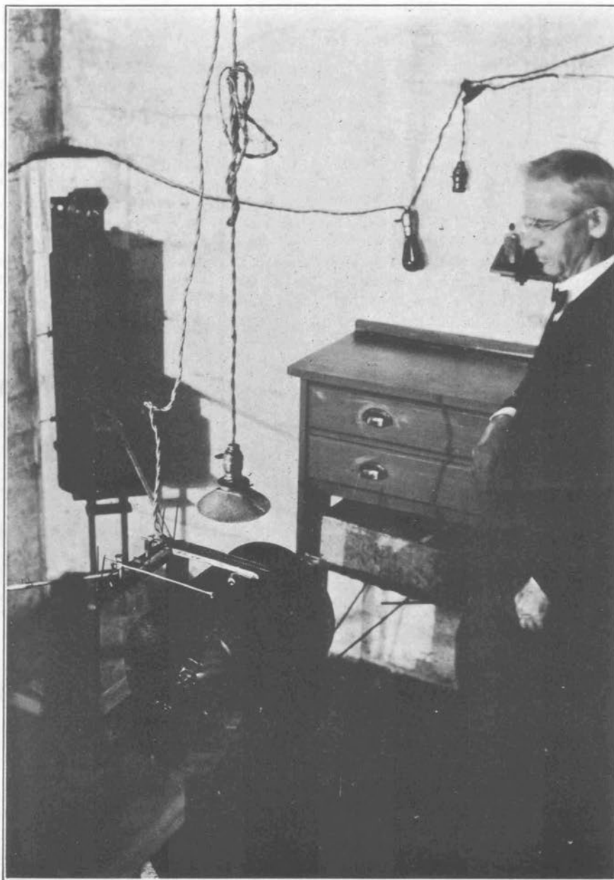
Interior of seismograph cellar at St. Mary's School, Hilo, Hawaii, showing two-component seismograph hung on wall of chamber, with recording drum in middle of room.
