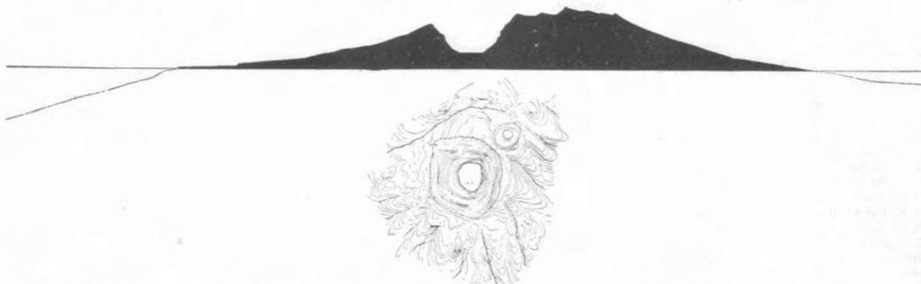
Profile section and map of Soufrière crater made by a sketch survey May 31, 1902, by T. A. Jaggar. Vertical and horizontal scales the same, 0.64 mile to the inch. Bottom of crater 2550 feet below summit, 1660 feet below rim. Diameter crater lip 4870 feet. Coast benches east 60 and 200 feet above sea level. Depth of ocean in profile 125 fathoms east, 530 fathoms west. Profile on line north 66 degrees east.
