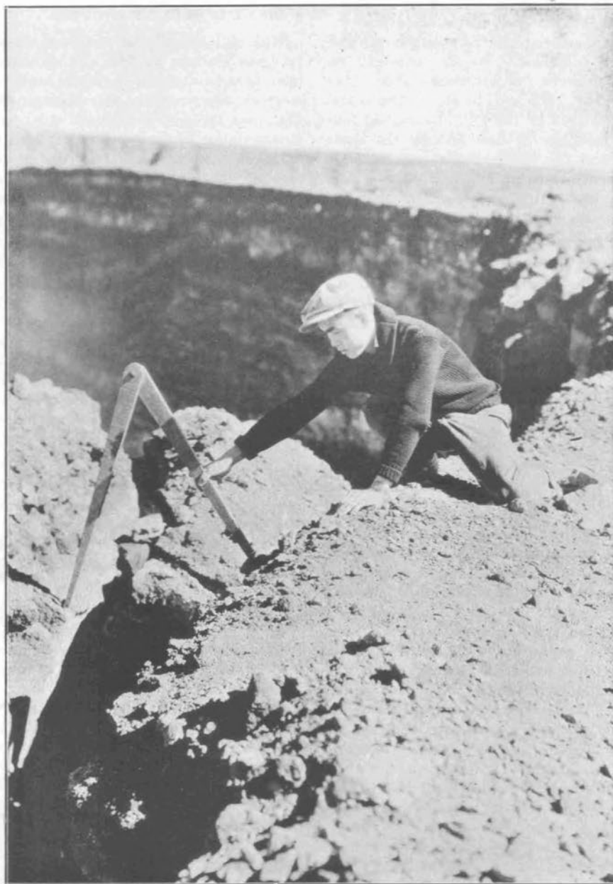
Marked crack where it emerges at southeast rim of Halemaumau, showing method of measurement with wooden calipers at painted spots.
