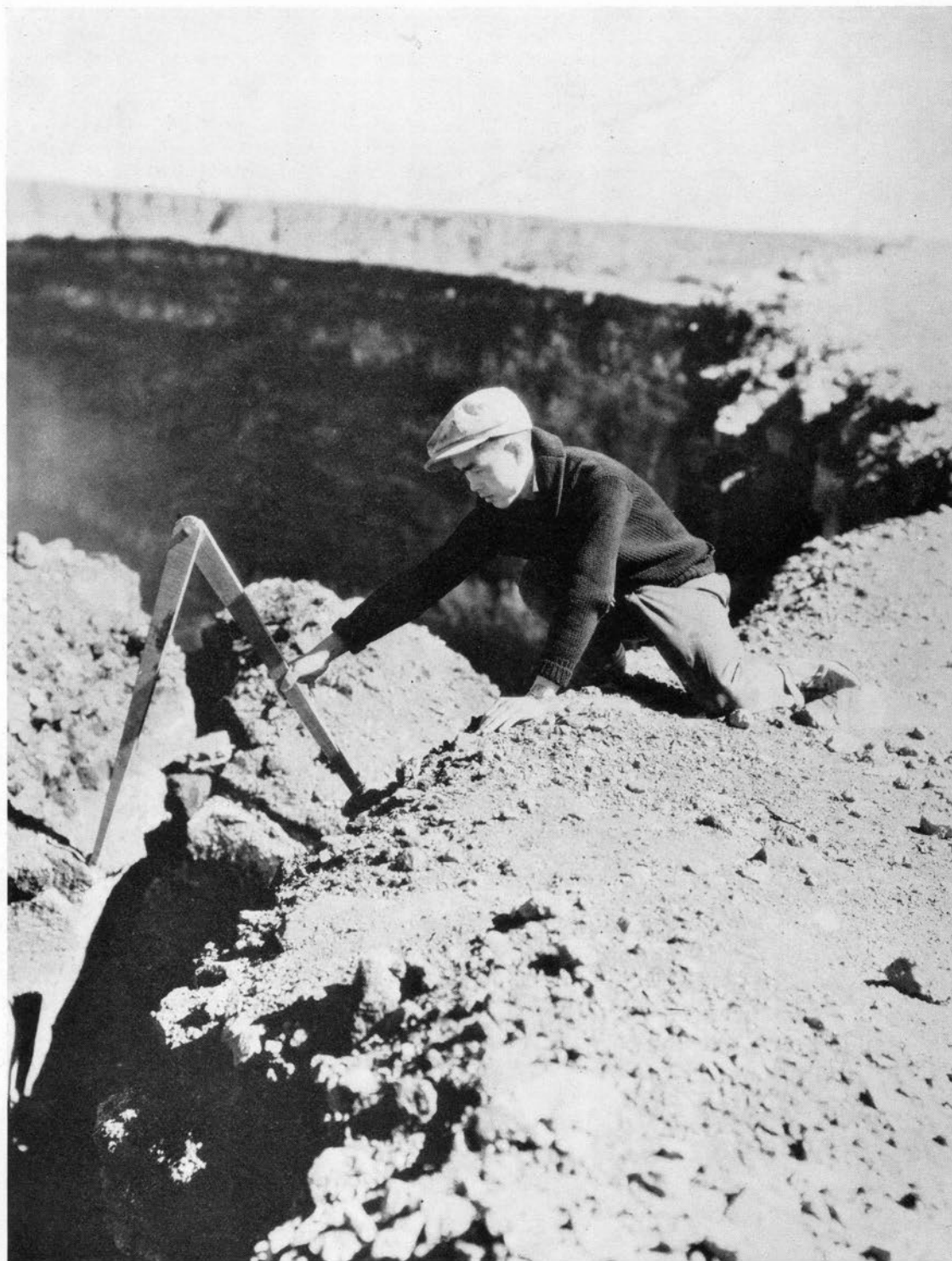
Use of caliper for measuring large cracks at Halemaumau. The crack is equipped with copper studs and, after setting, the caliper opening is measured with steel tape. An improved caliper is made with arc and clamp.
