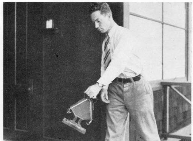
Weather Recording: Swinging wet-bulb and dry-bulb thermometers for relative moisture content of the air.
