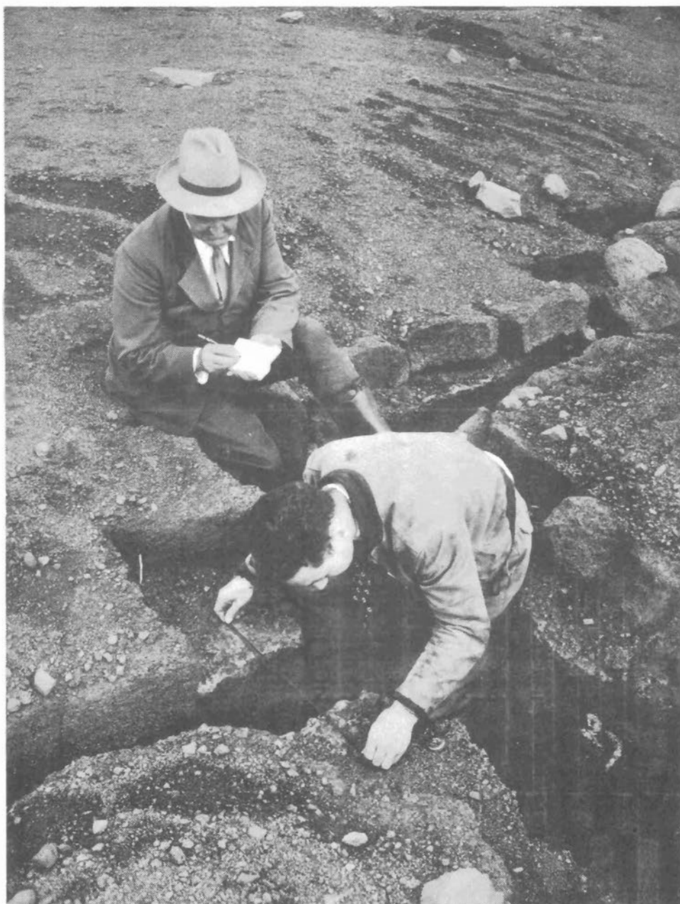
Measuring a crack locality on Halemaumau rim with steel tape over permanent metal studs in the rock.
