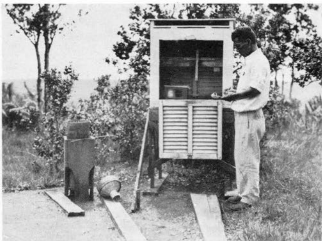
Weather Recording: Thermograph, rain gauge, maximum thermometer, minimum thermometer.
