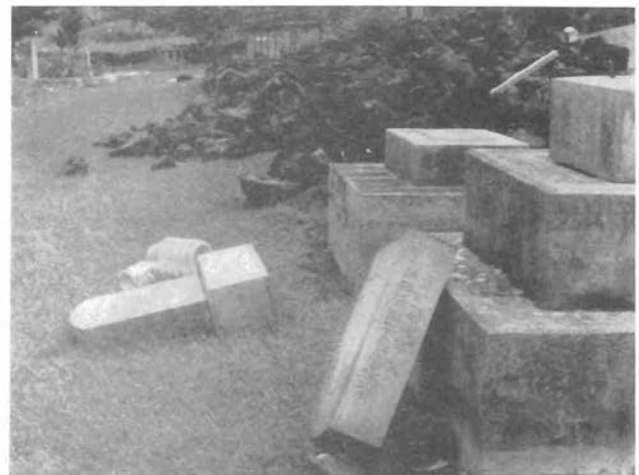
FIGURE 5. Overturned headstones in the cemetery of the Central Kona Church at Kealahakua were thrown westward from their foundations, but the base plate beneath the headstone in the foreground was shifted 2 inches eastward.
