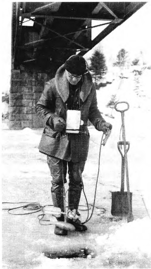
Stream flow measurement under ice-cover East Branch of the Penobscot River at Grindstone March 5, 1932
