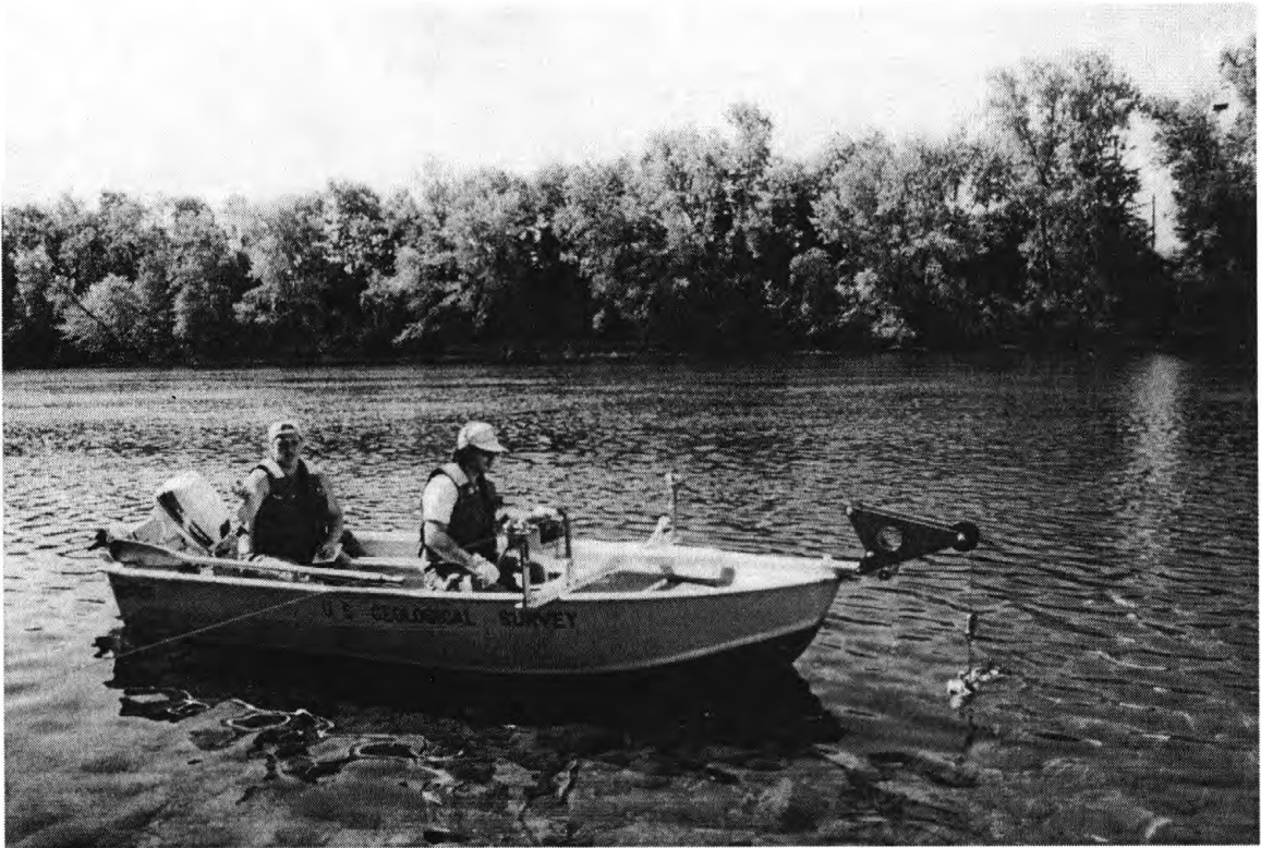
Streamflow discharge measurement from boat, Connecticut River at Montague City, Mass.
