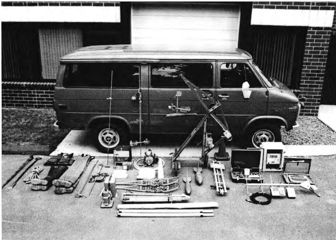
Typical complement of streamgaging equipment carried in USGS field vehicles.
