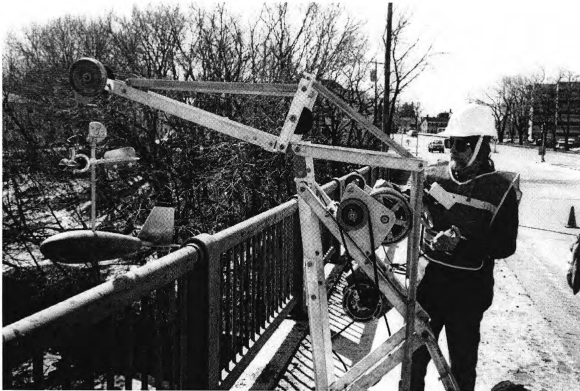
Hydrologic Technician Donald Searles uses 100-pound weight and electric reel to measure high flows in the Blackstone River at Northbridge, Massachusetts during a high-water event in March 1993.
