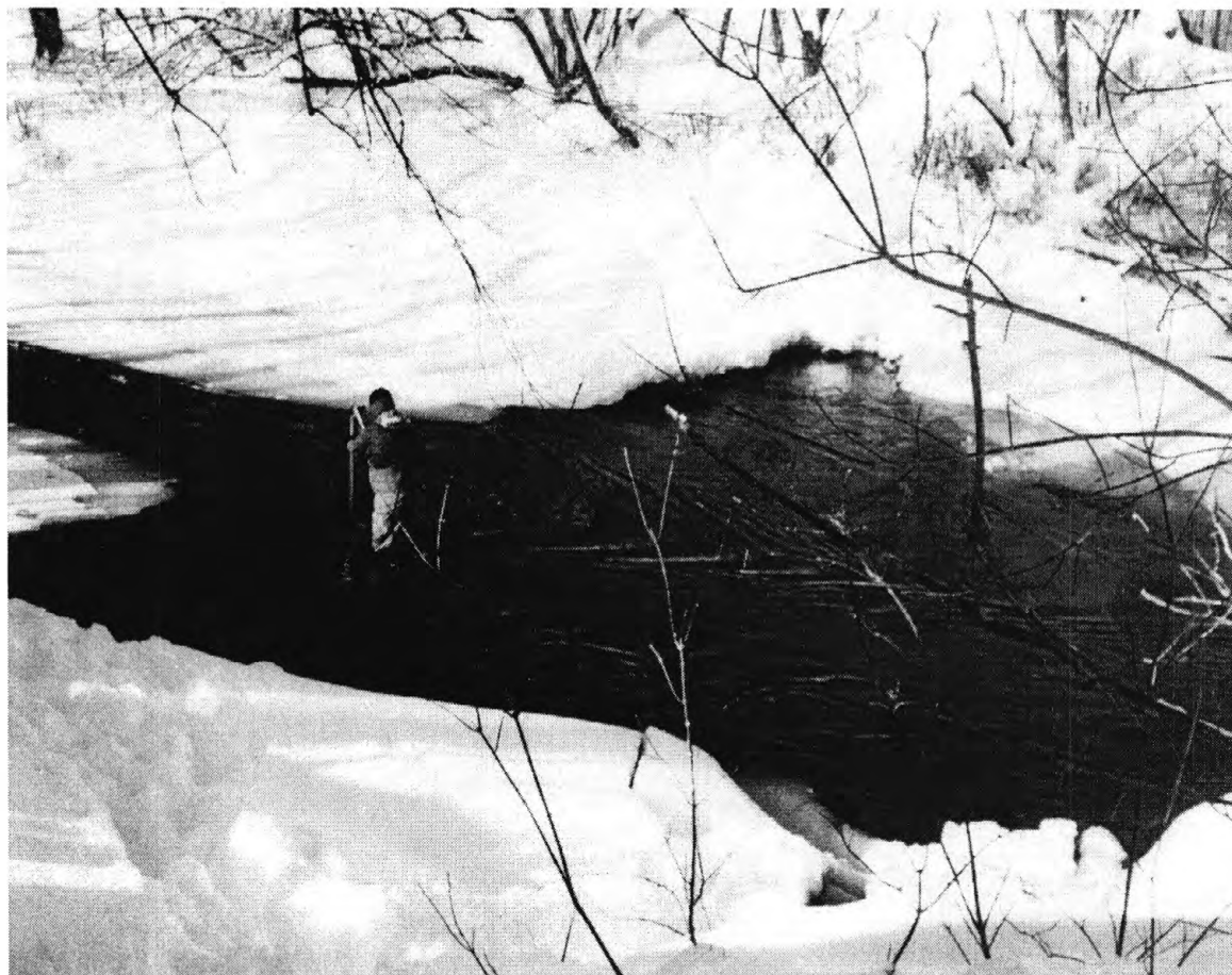
Hydrologic Technician R. Glenn Casey measures winter streamflow at Assabet River at Maynard, Massachusetts. Ice has been cut away to provide open area for measurements.
