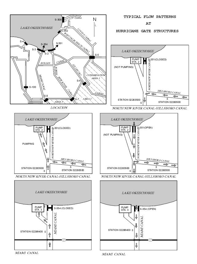
Figure 18. Typical flow patterns at Lake Okeechobee Control Structure.
