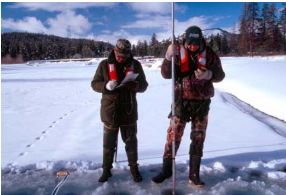
Winter discharge measurement under ice cover at Pacific Creek near Moran, Wyoming in the upper Snake River basin.
