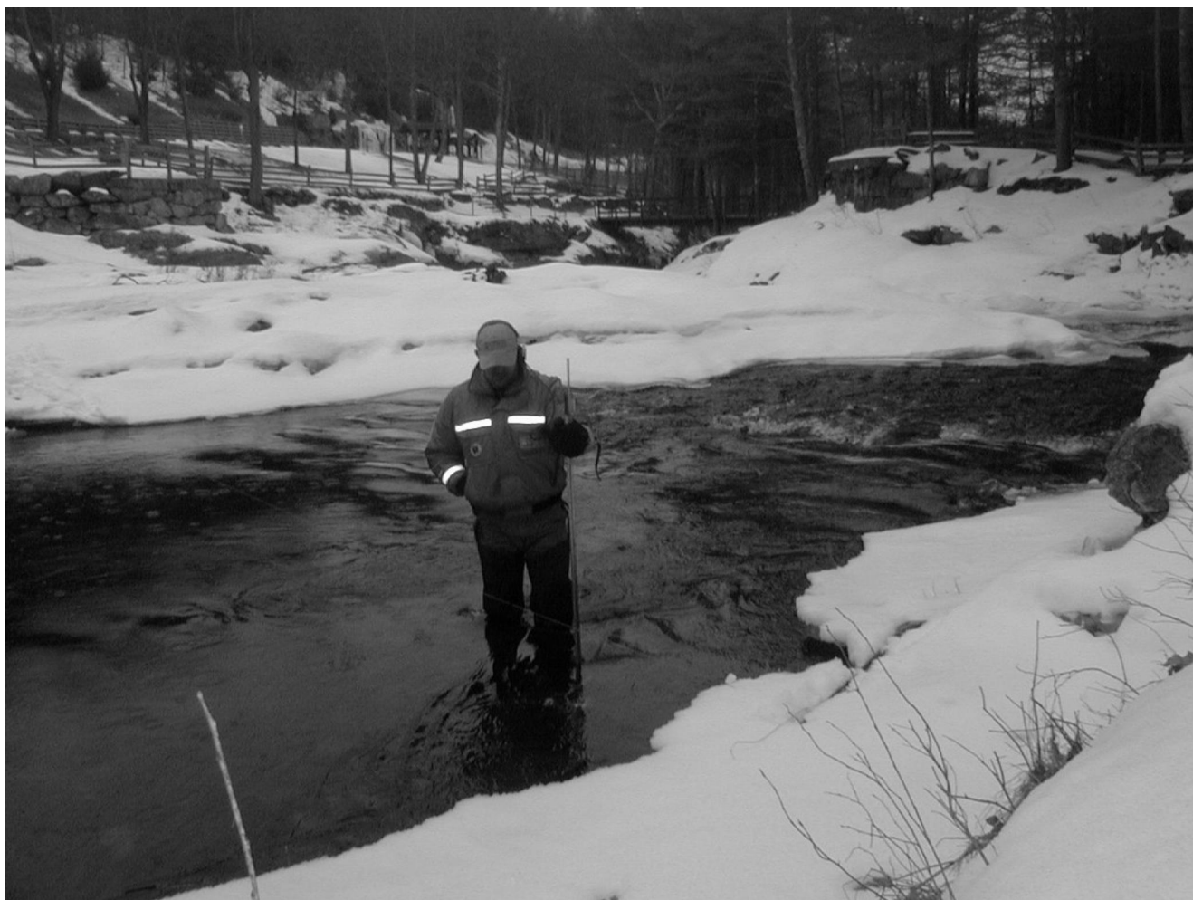
Wading discharge measurement Little Androscoggin River near South Paris (01057000) February 2005
