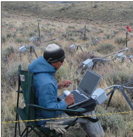
Figure 1. David Kesonie (USGS) downloading data from mantis sensors near the Fall Creek elk feedground, Pinedale, Wyoming. The "mantis" near-surface sensor platform (developed by Heidi Steltzer, Fort Lewis College, and others) has downward-facing sensors (for visible and near-infrared light) for measuring greenness in approximately 1 square meter and an upward-facing sensor for monitoring cloud cover. Reflectance and incoming solar radiation data were collected with 21 platforms from May 1 to September 1, 2010. Each site also had sensors to record air temperature and soil moisture 5 centimeters below the surface. Photograph by Geneva Chong, U.S. Geological Survey.
