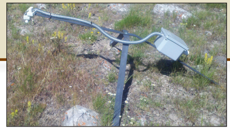
Figure 3. A mantis near-surface sensing platform with downward- and upward-facing sensors and the utility box, which contains the HOB0 data logger (Onset Computer Corporation), circuitry and battery pack. The system is weatherproof through growing season conditions, and the platform alone was stable left out through the winter (protected from cattle with solar electric fence). The greenness sensors are centered on a patch of cheatgrass ( Bromus tectorum ), which is an invasive, nonnative of concern throughout the western US. The sensors measure reflectance from an approximately 1-square-meter area. Photograph by Geneva Chong, U.S. Geological Survey. (Any use of trade, product, or firm names is for descriptive purposes only and does not imply endorsement by the U.S. Government.)
