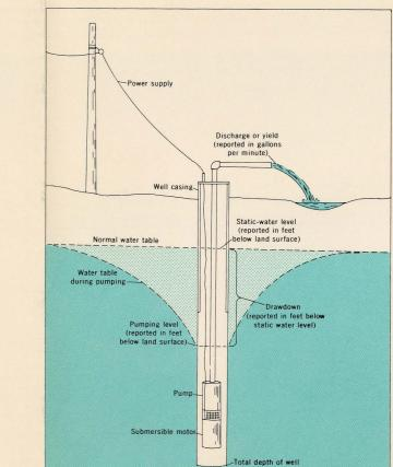
DIAGRAM OF TYPICAL WELL INSTALLATION
