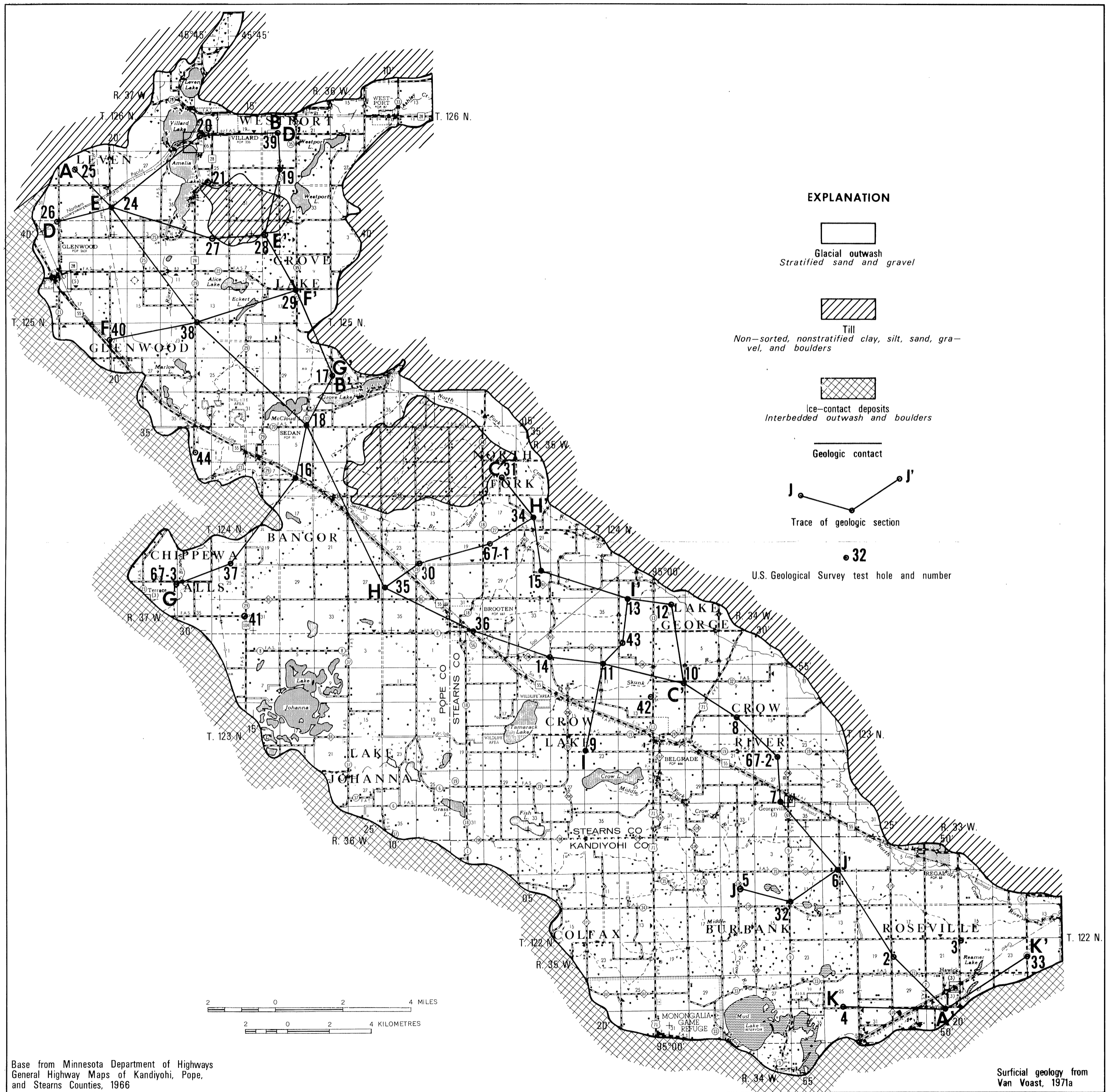
Plate 3.--Generalized surficial geology, location of test holes, and trace of geologic sections in the Brooten-Belgrade area.
