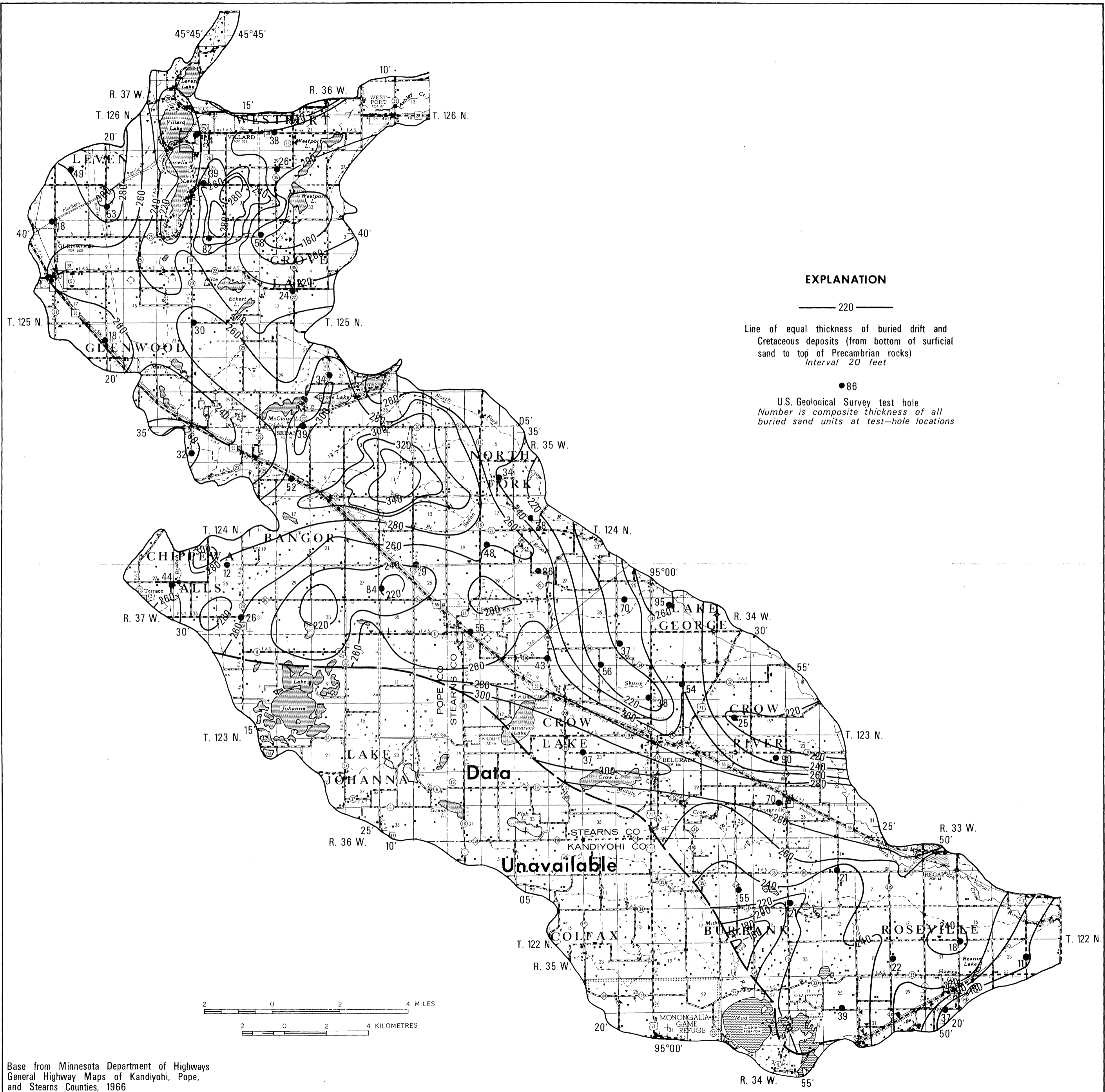
Plate 5.--Thickness of drift and Cretaceous deposits from bottom of surficial sand to top of Precambrian showing composite thickness of all buried sand units at test-hole locations.
