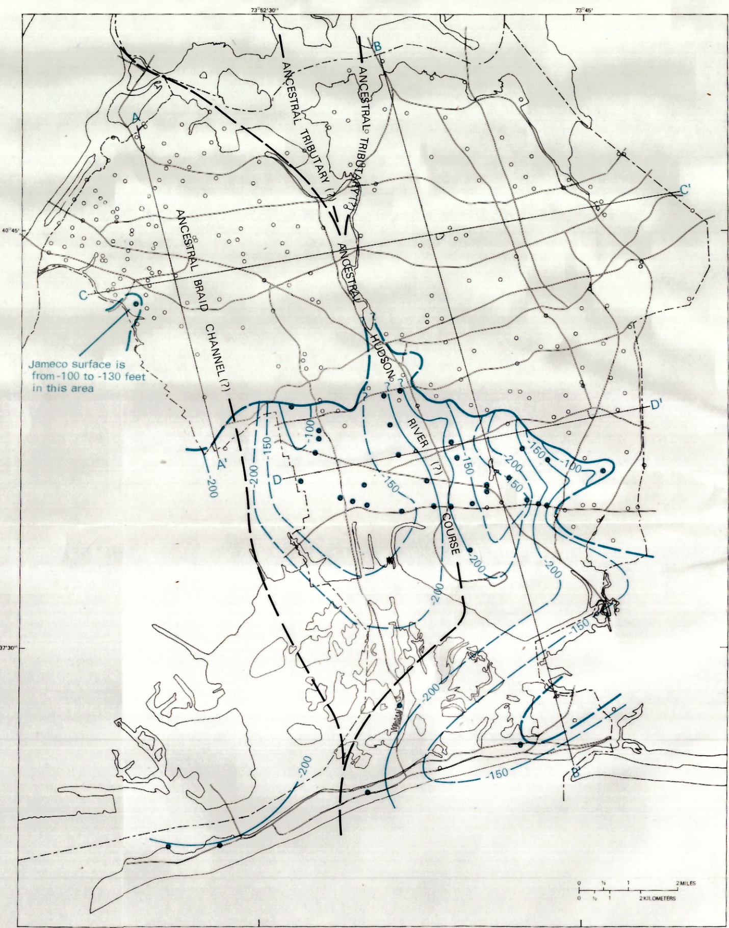
E. JAMECO GRAVEL SURFACE IN QUEENS COUNTY
