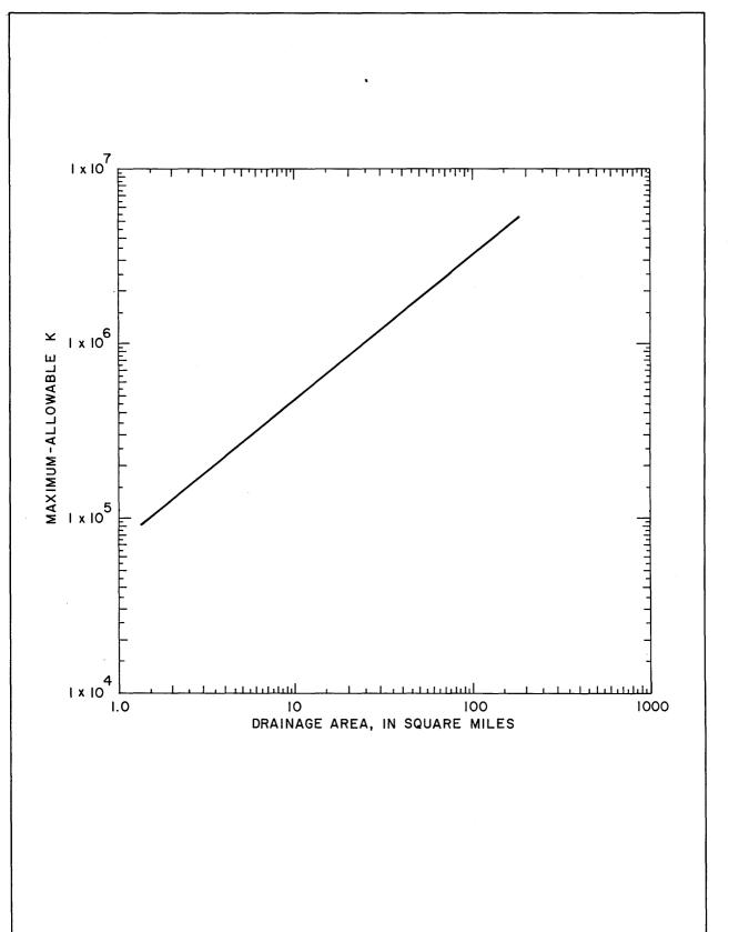
FIGURE 2.-Maximum allowable conveyance versus drainage area
