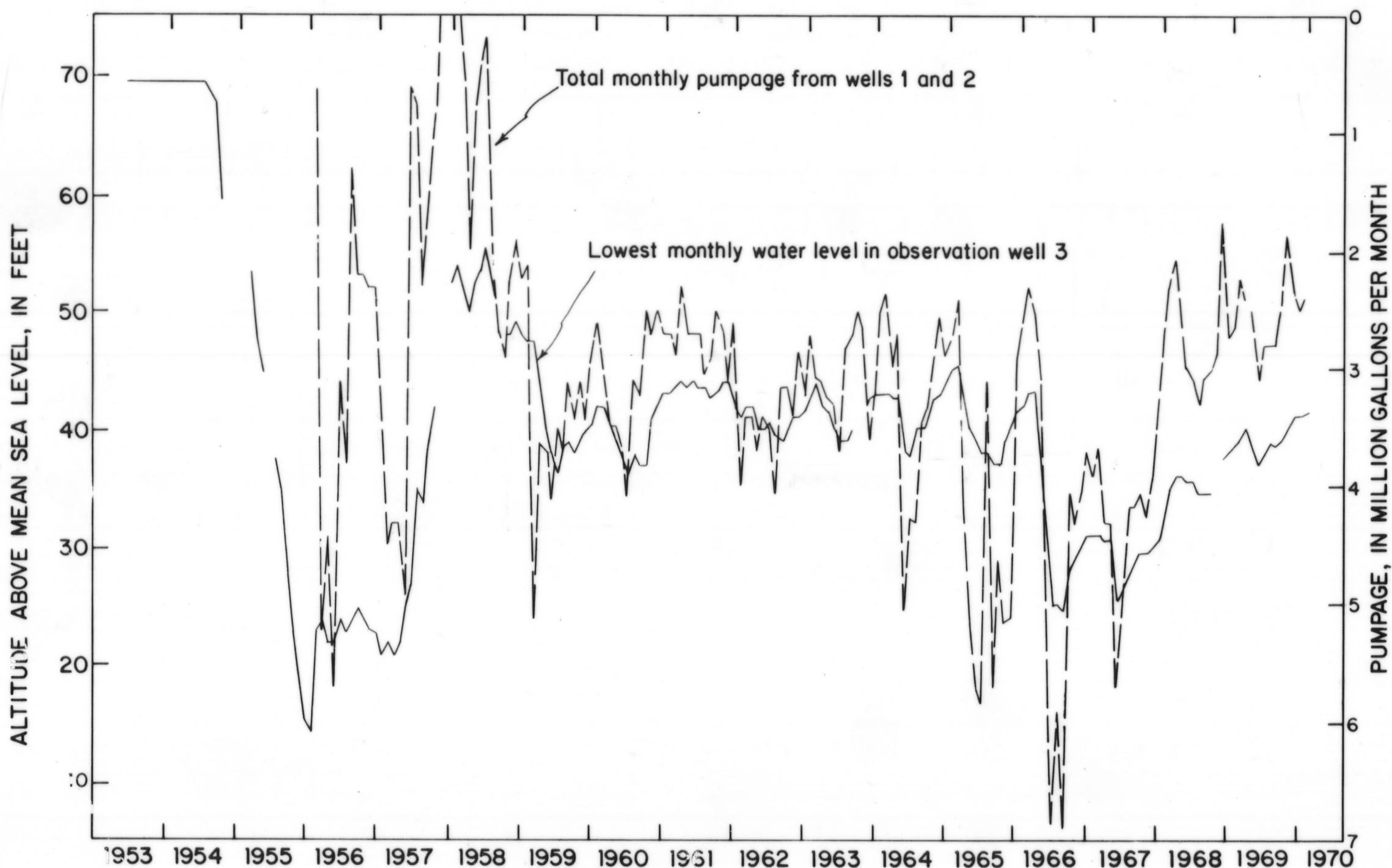
**Figure 45. — Effects of pumping on water-level fluctuations in the Ancora State Hospital wells tapping the Vincentown and Manasquan Formations undifferentiated, 1953-70.**
