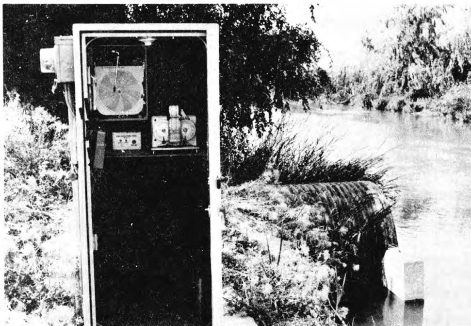
Figure 4.—Variable-backwater-streamflow-gaging station at Twenty-First South Conduit at Jordan River. Depth and velocity of flow in conduit monitored by Marsh McBirney, Inc., Model 250 velocity-modified flowmeter and recorded as discharge on circular chart and Fisher Porter digital tape.
