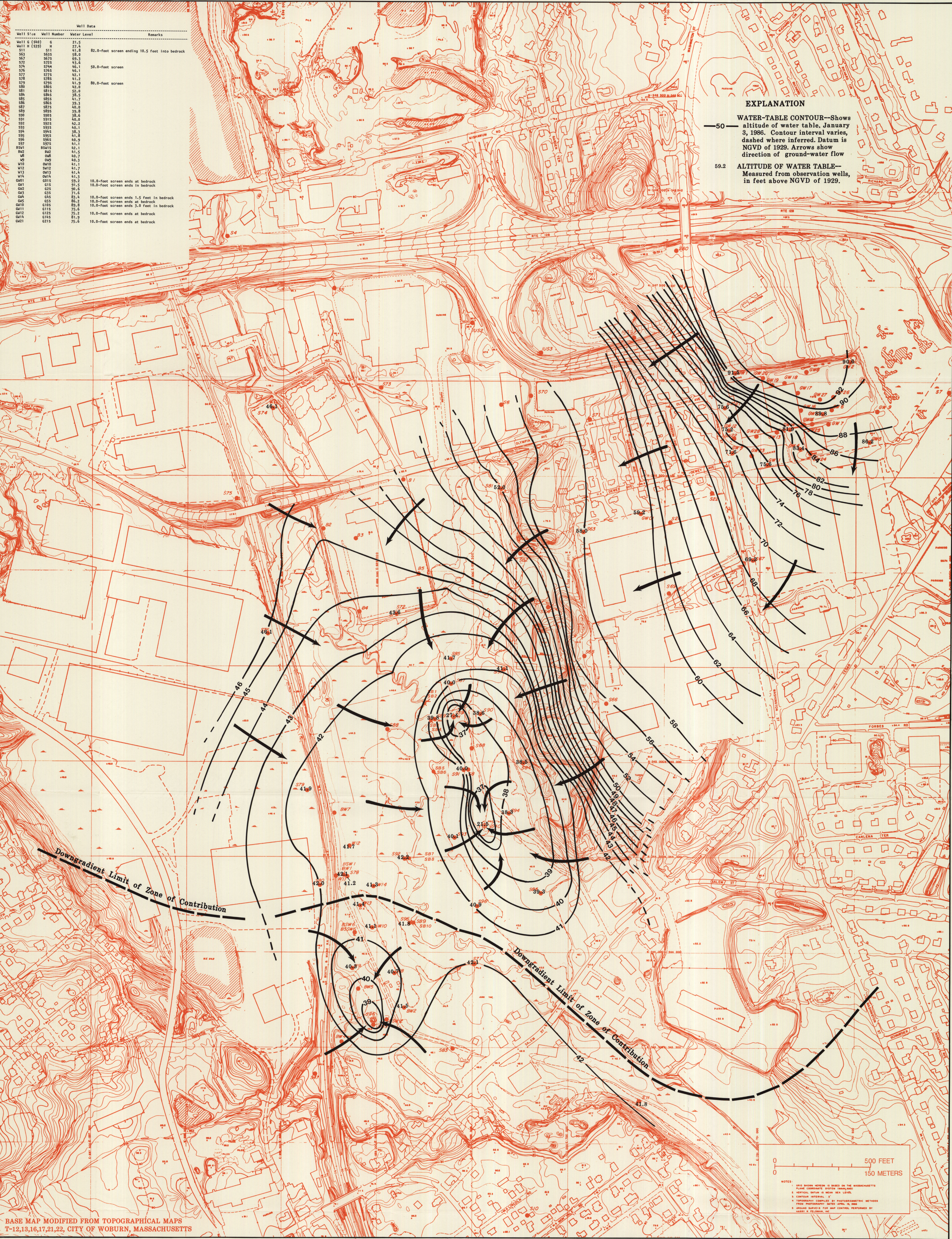
Altitude of the water table after 30 days of pumpage from wells G and H, January 3, 1986
