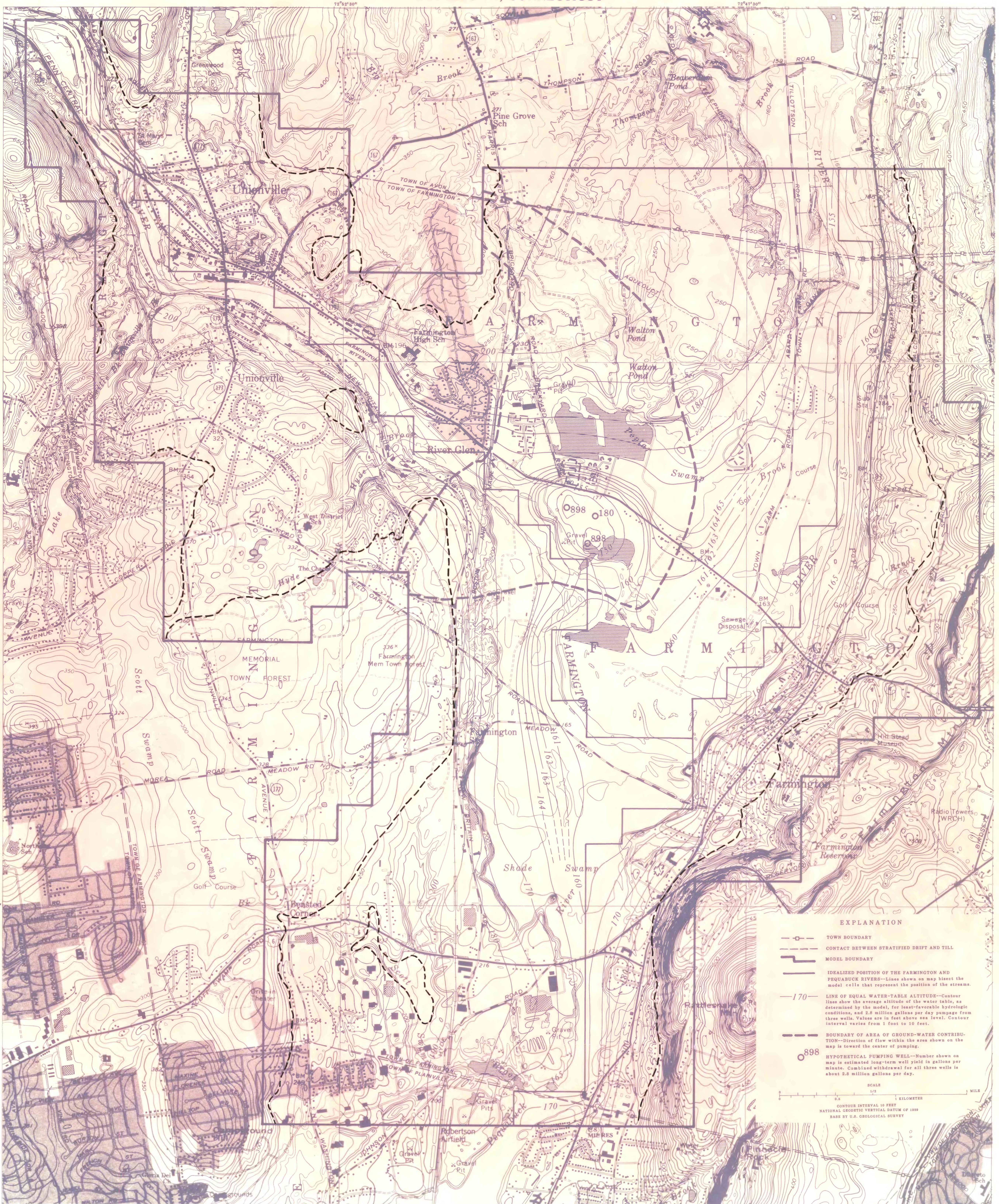
SIMULATED WATER-TABLE ALTITUDE AND AREA CONTRIBUTING FLOW IN THE FARMINGTON AQUIFER, LEAST-FAVORABLE HYDROLOGIC CONDITIONS, 2.8 MILLION GALLONS PER DAY PUMPAGE
