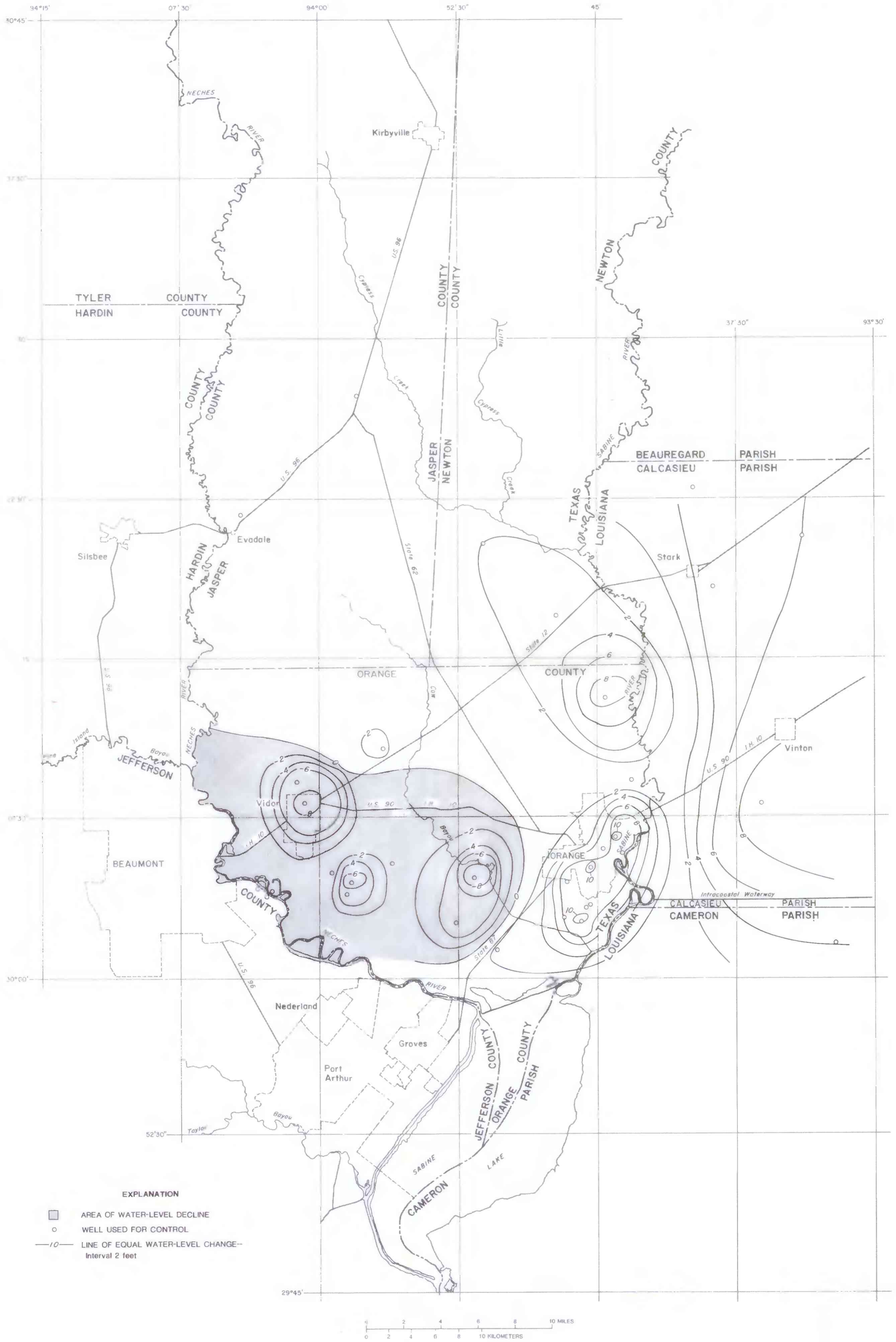
Figure 5.—Approximate change in water levels in wells screened in the lower unit of the Chicot aquifer, spring 1971 to spring 1985.
