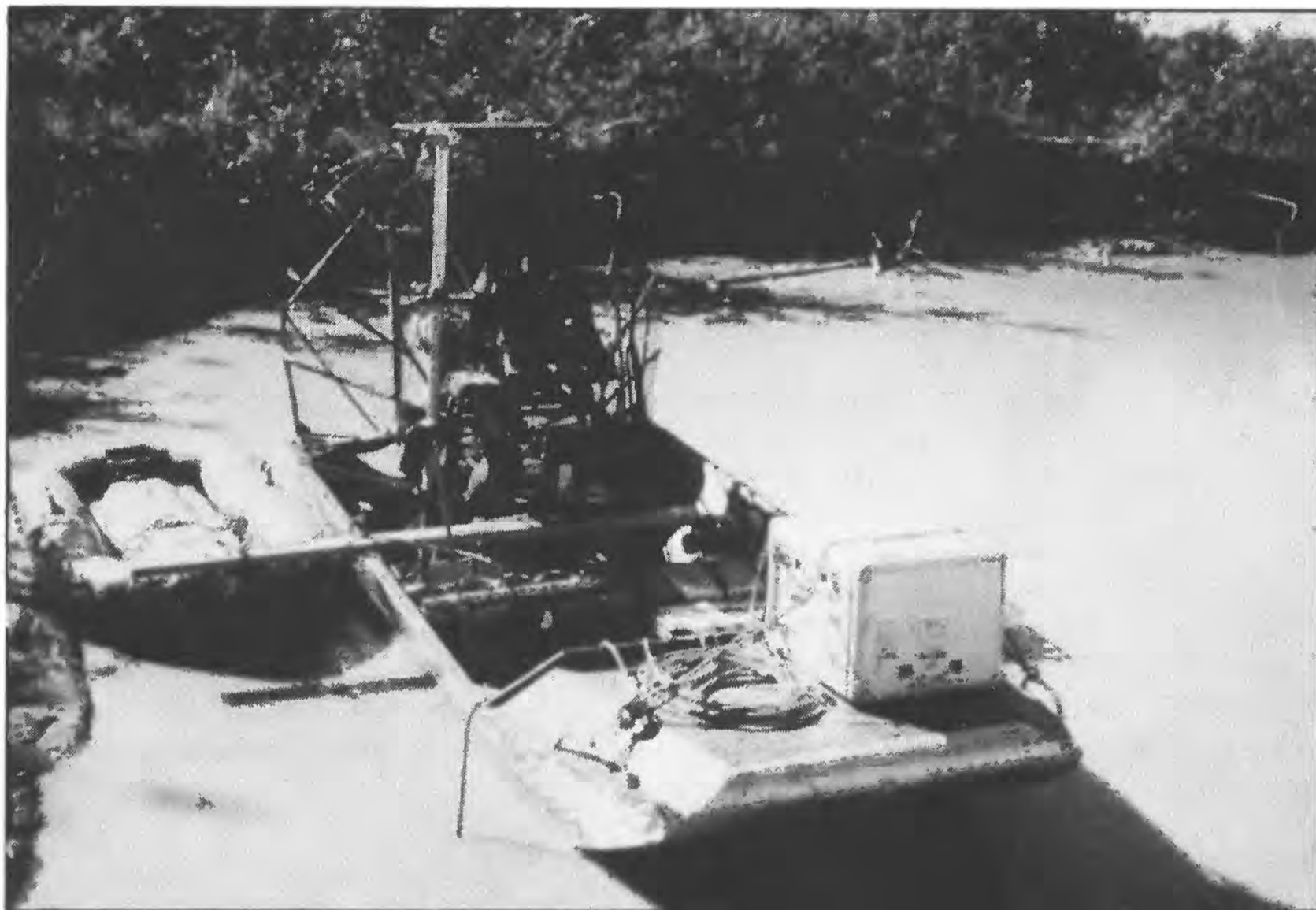
Figure 5. Airboat equipped with ground-penetrating radar.
