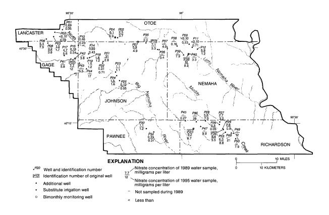
Figure 2. Nitrate concentrations in water from sampled wells in the paleovalley alluvial aquifers, Nemaha Natural Resources District, Nebraska, 1989 and 1995.
