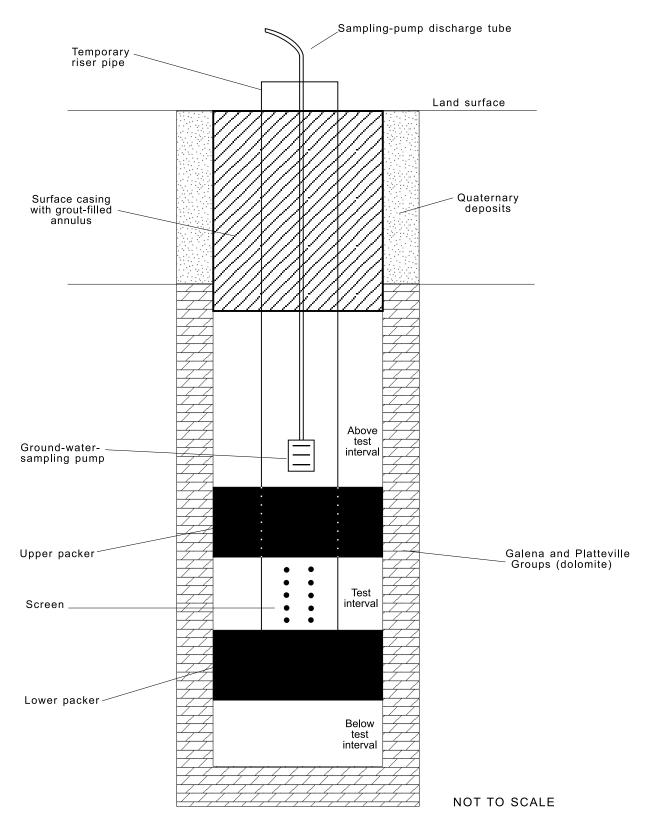
Figure 8. Packer assembly and ground-water sampling pump in a borehole.
