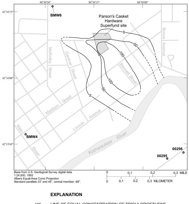
—100-- LINE OF EQUAL CONCENTRATION OF TRICHLOROETHENE--Contour interval, in micrograms per liter, is variable. Dashed where inferred
