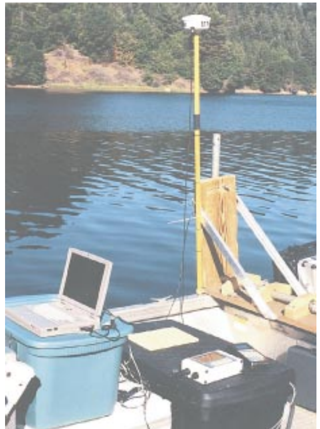
Figure 3. Depth-sounding equipment and global positioning system (GPS) used to survey the topography of Loch Lomond Reservoir in Santa Cruz County, California.
