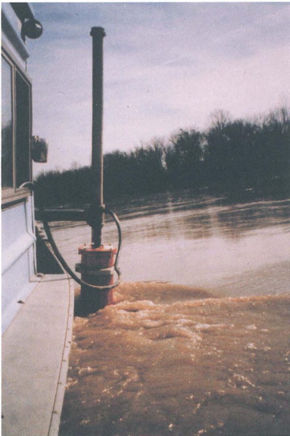
Measuring discharge on the Yazoo River using a boat-mounted acoustic Doppler.
