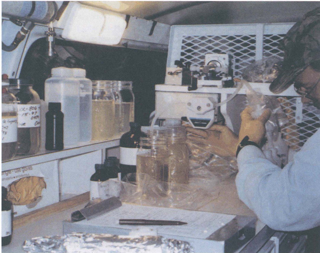
Water samples were filtered and processed in a mobile laboratory immediately after sample collection.
