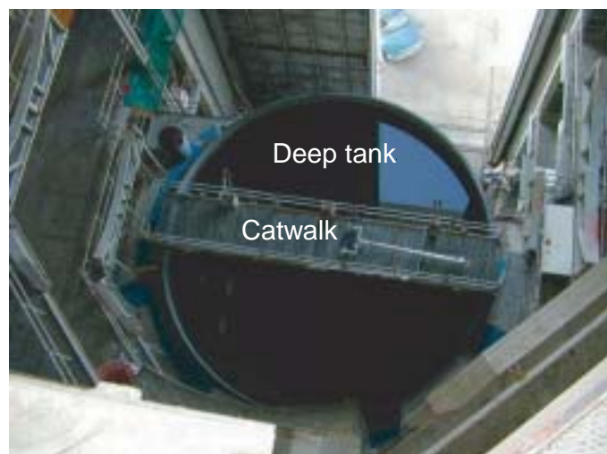
Figure 23. Photographs of tow tank and tow cart (top) and deep tank (bottom) at the U.S. Geological Survey Hydraulics Laboratory, Stennis Space Center, Mississippi.
