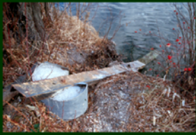
Staff gage undercut by bank erosion
