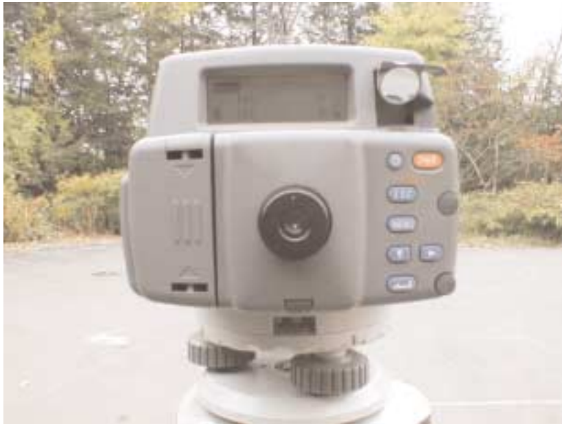
Figure 2. User end of level includes display screen, leveling mirror, battery compartment (on left), eyepiece, and user buttons.
