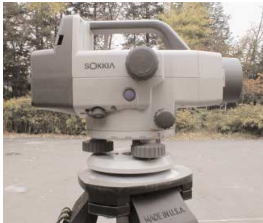
Figure 3. Side view of level displays focus and rotate knobs and measure button.
