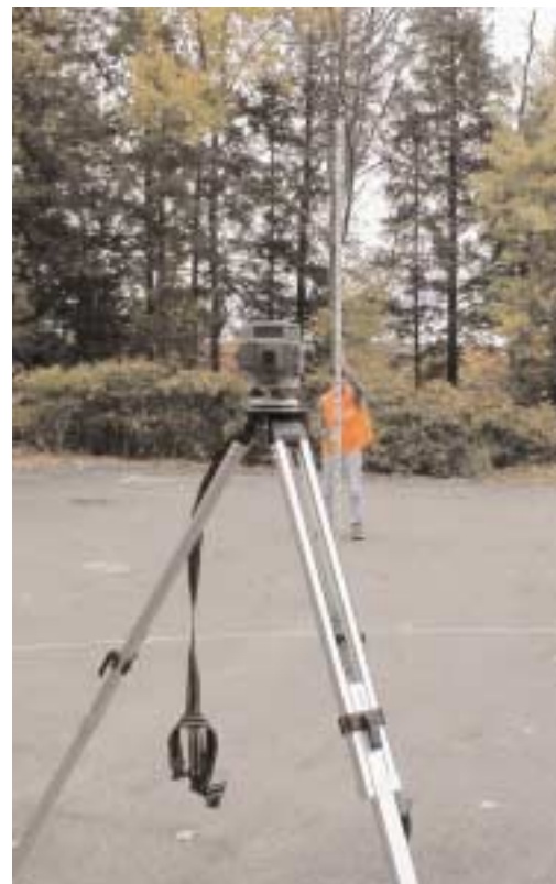
Figure 1. Digital level on standard tripod reading bar-coded rod.
