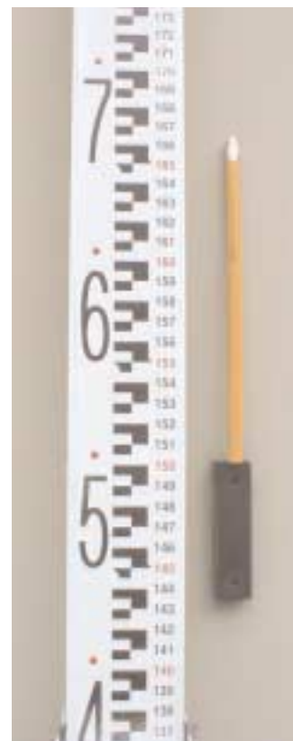
Figure 5. Metric graduations on rod to be read by eye.
