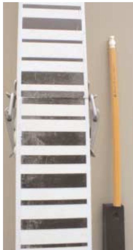
Figure 6. Bar-coded side of rod and buckles.
