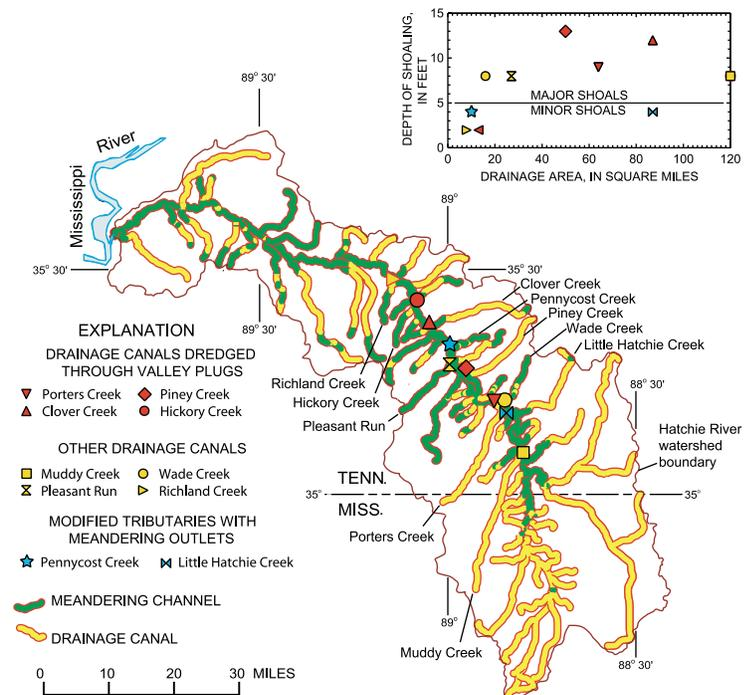
Figure 3. Shoals of the Hatchie River and drainage area of shoal-producing tributaries.
