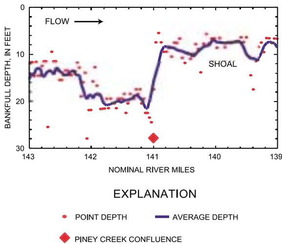
Figure 2. Depth profile of the Hatchie River bed at Piney Creek, in Tennessee.
