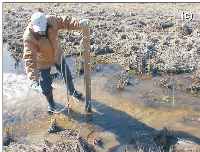
Figure 5. (a) Mini-piezometer installation in the bed of Pipe Elm Branch, (b) mini-piezometer screen, and (c) manometer used to measure relative ground-water and surface-water levels, Dover Air Force Base, Delaware.
