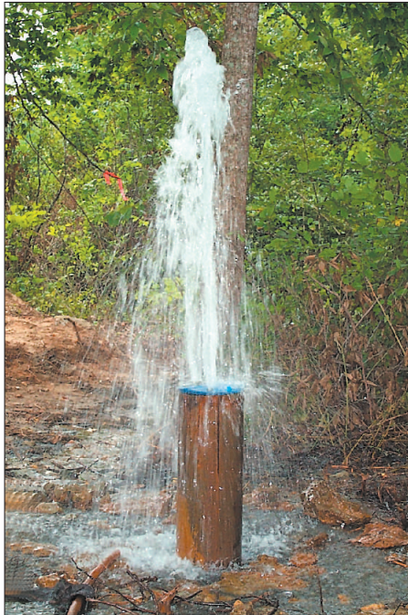
Flowing artesian wells, like 14FF59 shown above, are commonly found in areas that are topographically lower than the adjacent recharge area. This well flows about 40 gal/min out of two 1-inch openings through the blue pressure cap installed at the top of casing, and about 50–60 gal/min when left uncapped. The top of the stream of water is about 5.5 feet above land surface. (Photo by Randy Kath, State University of West Georgia.)
