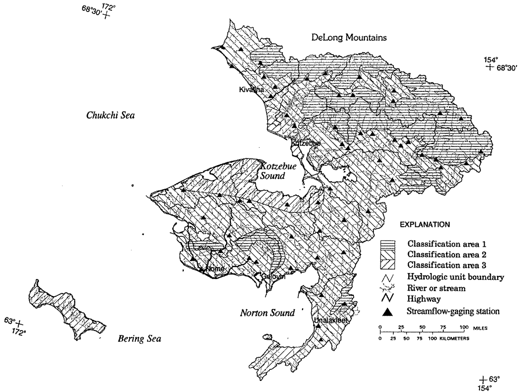
Figure 14. Proposed streamflow-gaging network and classification areas for Northwest Alaska.
