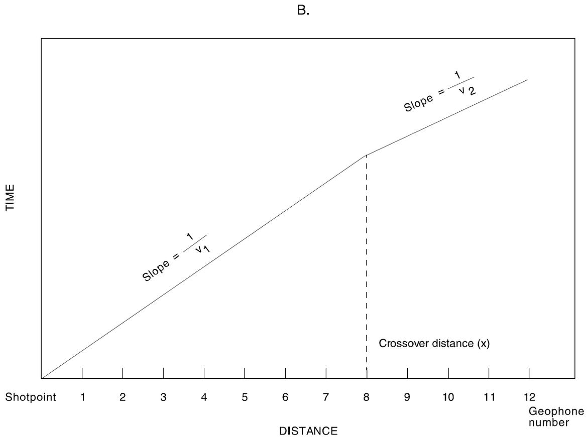
**Figure 3.** Diagrams showing (A) sound-wave propagation in unsaturated and saturated zones and detection at land surface, and (B) the corresponding time-distance curve. (Modified from Haeni, 1988, fig. 2.)
