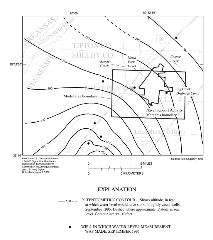
**Figure 13**. Altitude of the potentiometric surface of the Memphis aquifer in northern Shelby County near Naval Support Activity Memphis, Millington, Tennessee.
