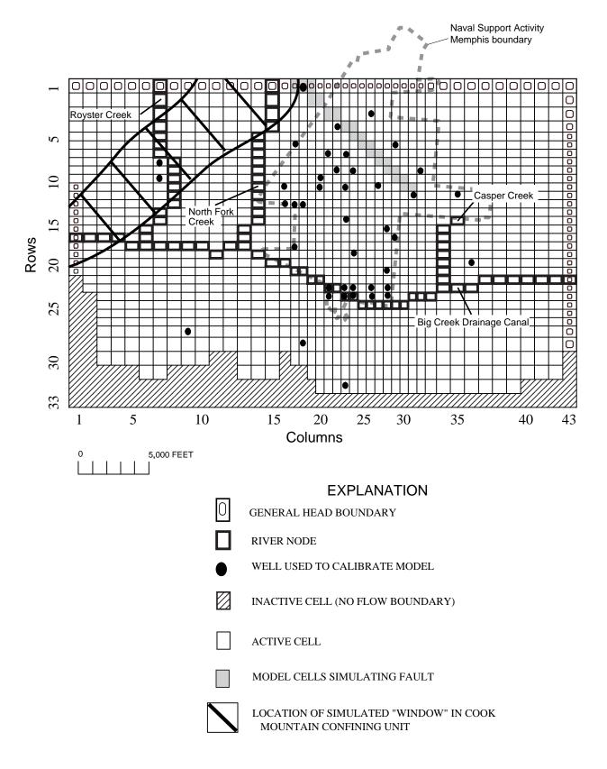
**Figure 17**. Model grid, wells used to calibrate model, cells simulating fault, location of a simulated window in Cook Mountain confining unit, and boundary conditions for the flow model of the shallow aquifer system in the area of Naval Support Activity Memphis, Millington, Tennessee.
