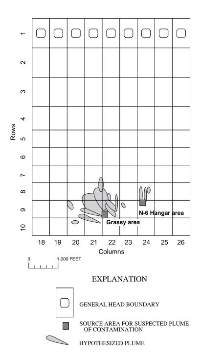
**Figure 25**. Locations of selected hypothesized plumes of contamination in the alluvial-fluvial deposits aquifer at two sites within the Norhside Area of Concern at Naval Support Activity Memphis, Millington, Tennessee (Source: EnSafe, written commun., 1997).
