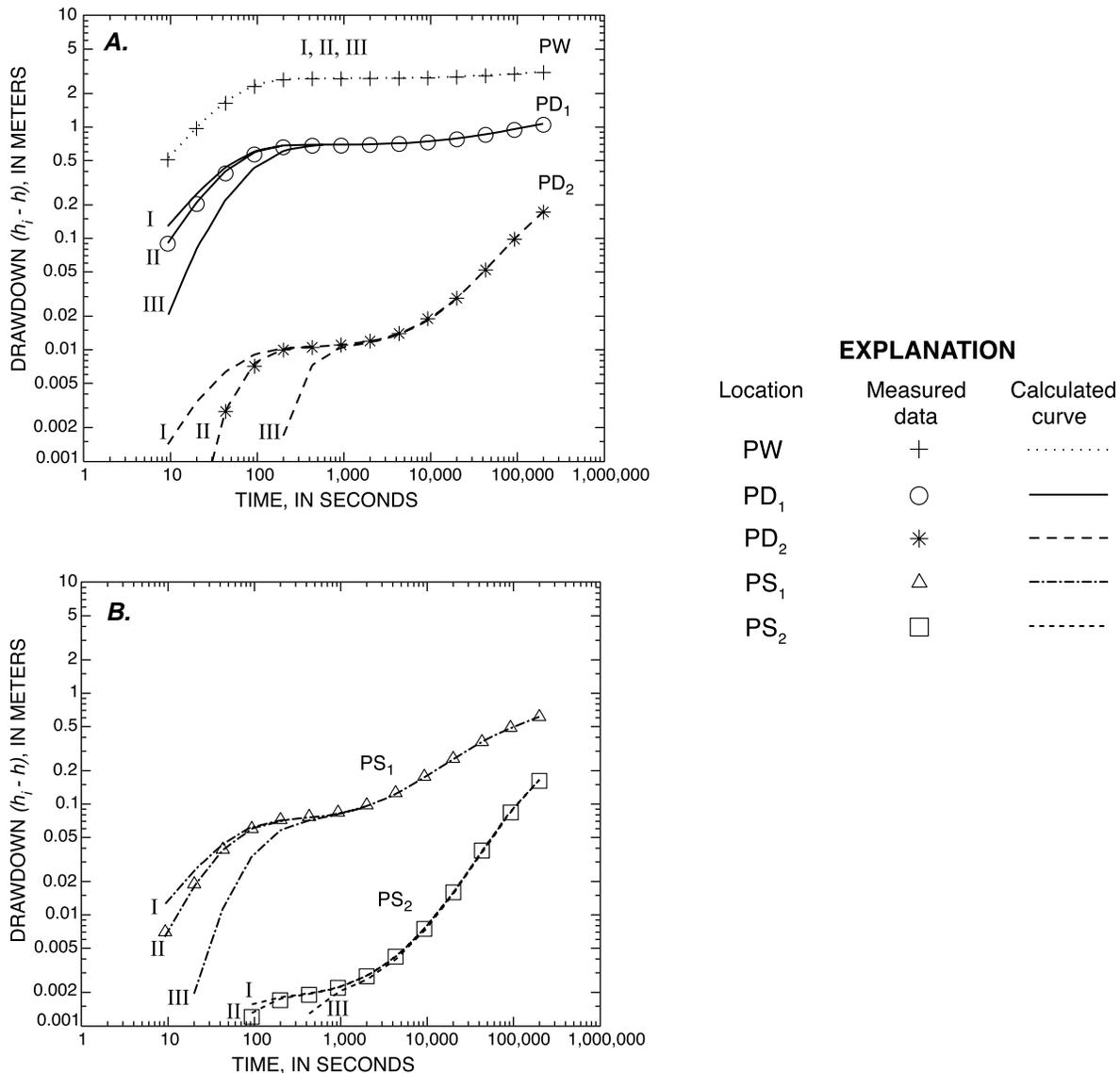
**Figure 11.** Drawdown versus time for the hypothetical water-table aquifer. Calculated curves use values of specific storage equal to  $2.0 \times 10^{-6} \text{ m}^{-1}$  (I),  $2.0 \times 10^{-5} \text{ m}^{-1}$  (II), and  $2.0 \times 10^{-4} \text{ m}^{-1}$  (III). (A) Wells PW, PD<sub>1</sub>, and PD<sub>2</sub>. (B) Wells PS<sub>1</sub> and PS<sub>2</sub>.
