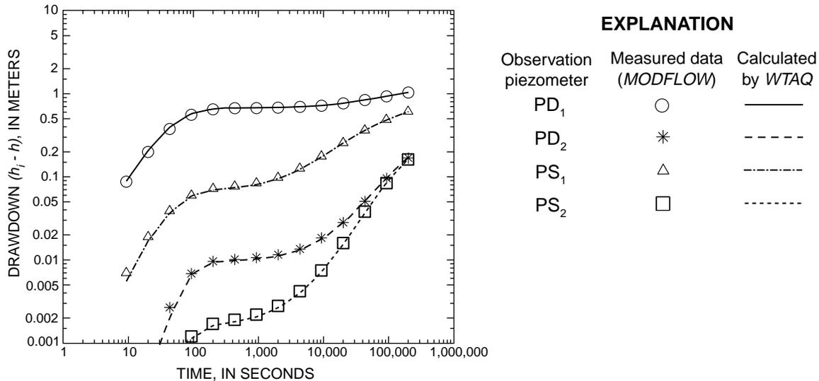
**Figure 12.** Drawdown versus time at the four observation piezometers for the hypothetical water-table aquifer. Drawdowns calculated by *WTAQ* using estimated values of hydraulic properties (lines) and by *MODFLOW* using true values of hydraulic properties (symbols).
