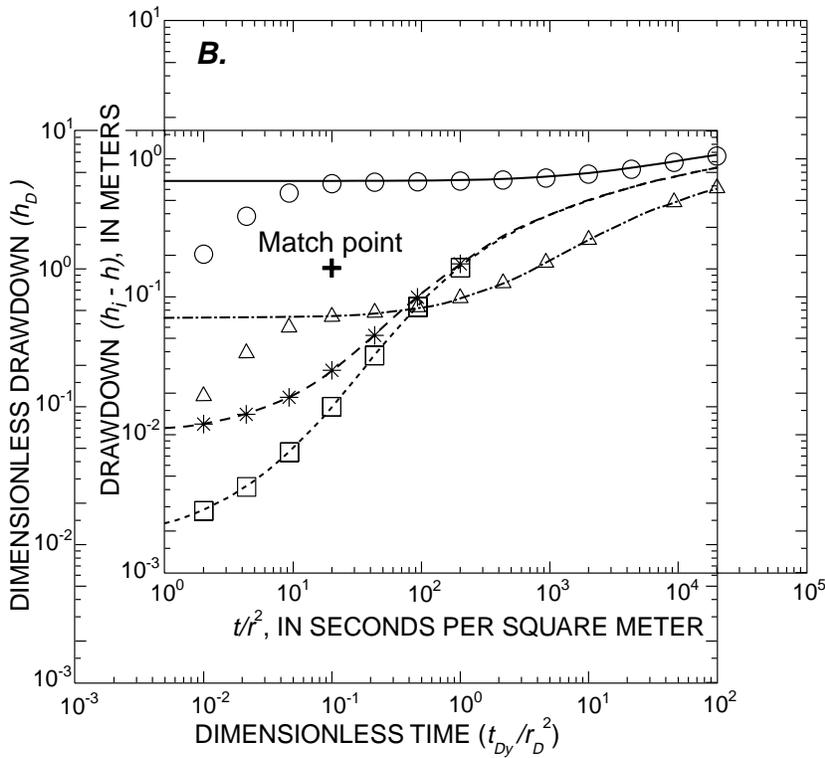
**Figure 10.** Composite plots of measured drawdown ( $h_i - h$ ) and calculated dimensionless drawdown (type curves) for (A)  $K_D = 0.1$  and (B)  $K_D = 0.5$  for the hypothetical water-table aquifer. ( $K_D$ , ratio of horizontal to vertical hydraulic conductivity;  $t/r^2$ , time divided by the square of the radial distance of the piezometer from the axis of pumped well.)
