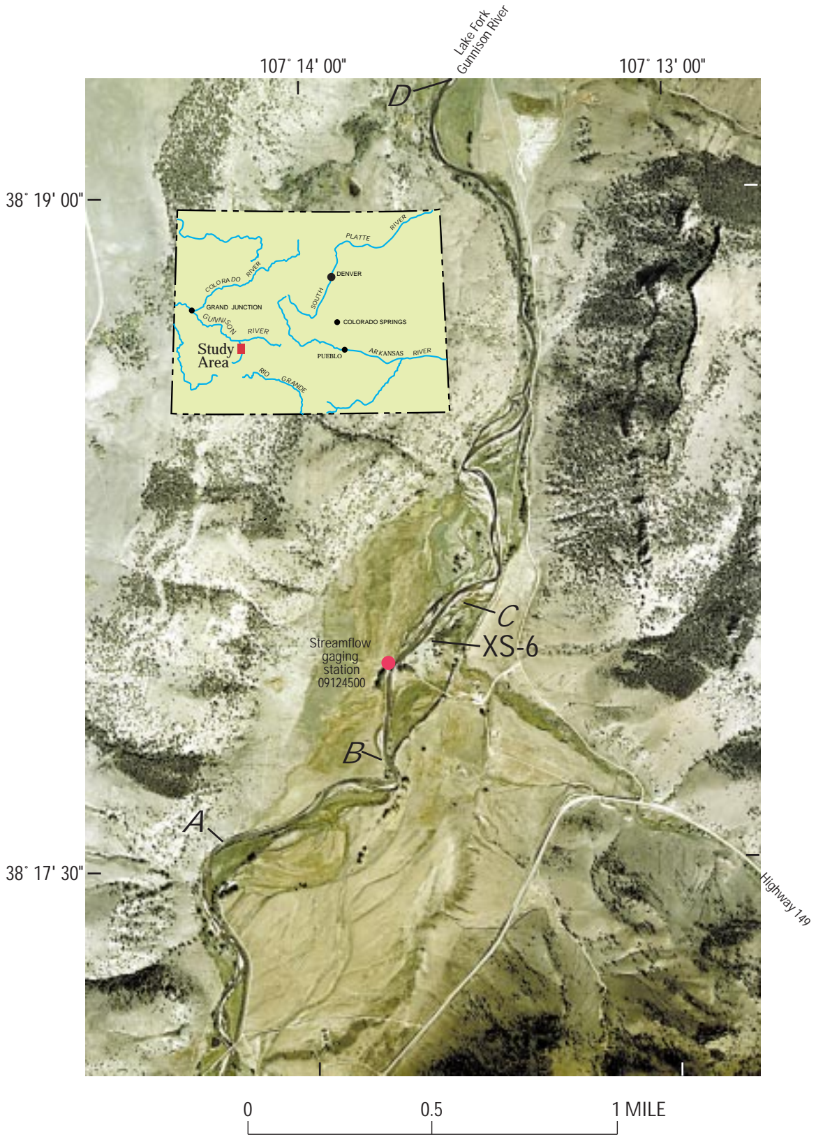
Figure 1. Aerial photograph of the Lake Fork of the Gunnison River at Gateview, Colorado, reach taken in 1977 before channel reconfiguration activities showing location of streamflow-gaging station 09124500, reach reconstructed in 1997 (A–D), and reach monitored by U.S Geological Survey in 1998 (B–C).
