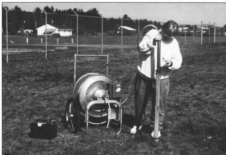
Figure 16. Typical setup for sampling water quality at a well in Concord, south-central New Hampshire.
