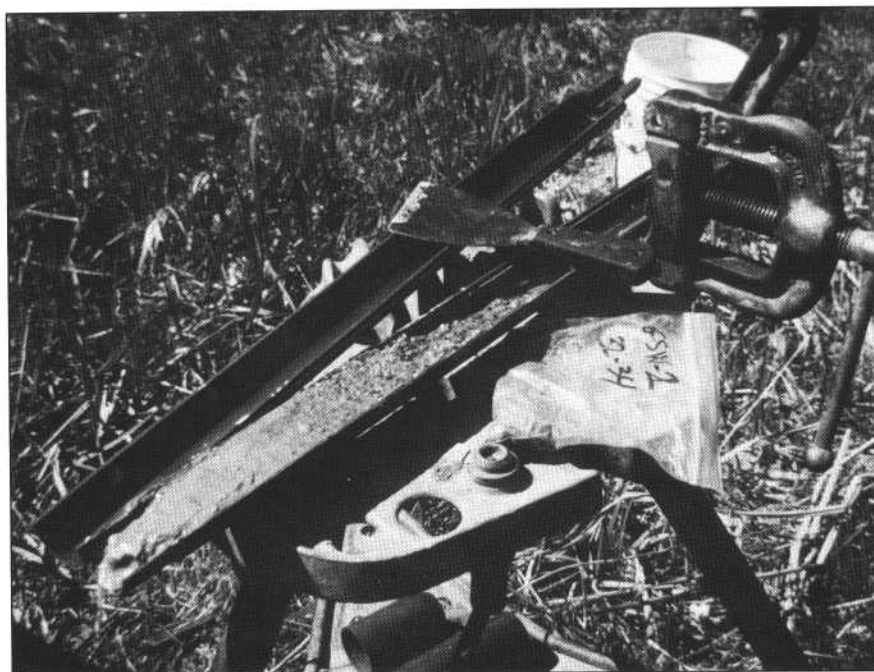
Figure 14. Split-spoon sampler and sediment from a drilled test hole. The sampler was used to retrieve aquifer material from drilled test holes and wells at 5- or 10-foot intervals. Once the sample is obtained, it is stored in the plastic bag for further analysis. (Photograph taken by J.D. Ayotte, U.S. Geological Survey.)
