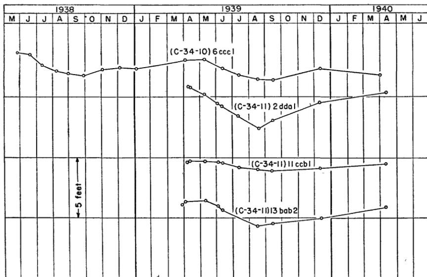
FIGURE 12.—Hydrographs of four shallow wells near Rush Lake showing effects of evaporation and transpiration.
