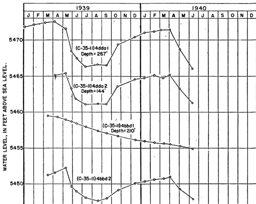
FIGURE 7.—Hydrographs of adjacent deep and shallow wells showing effects of pumping for irrigation.
