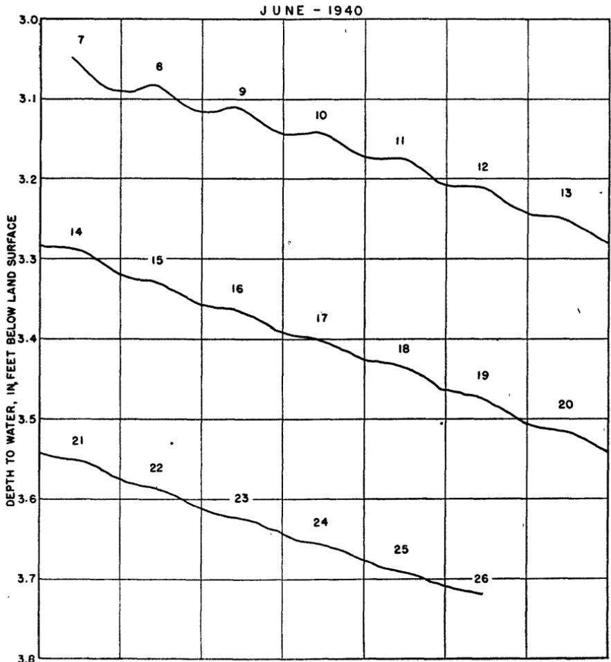
FIGURE 11.—Hydrograph showing daily fluctuations and general downward trend of water level in well (C-34-11)2bbd1.
