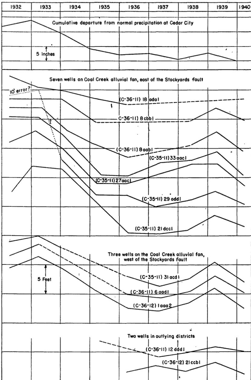
FIGURE 14.—Hydrographs showing approximate high-water levels each year in 12 wells in Cedar City Valley, 1932-40.
