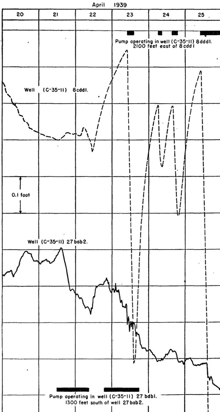
FIGURE 6.—Hydrographs of two wells in Cedar City Valley showing fluctuations caused by pumping in nearby irrigation wells.
