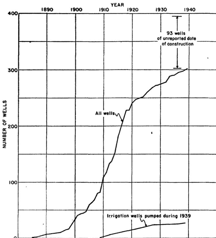
FIGURE 17.—Graph showing cumulative number of wells constructed in Parowan Valley, 1885-1939.
