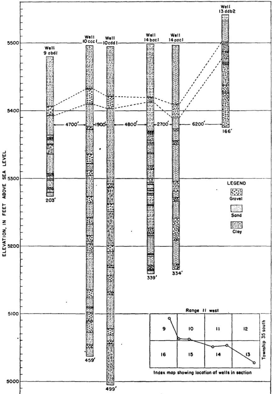
FIGURE 3.—Logs of six wells in Cedar City Valley and suggested correlations of the coarser sediments.
