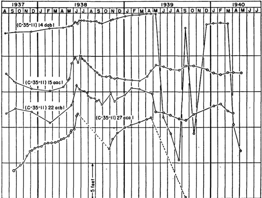
FIGURE 9.—Hydrographs of four wells near the eastern margin of the Coal Creek alluvial fan.
