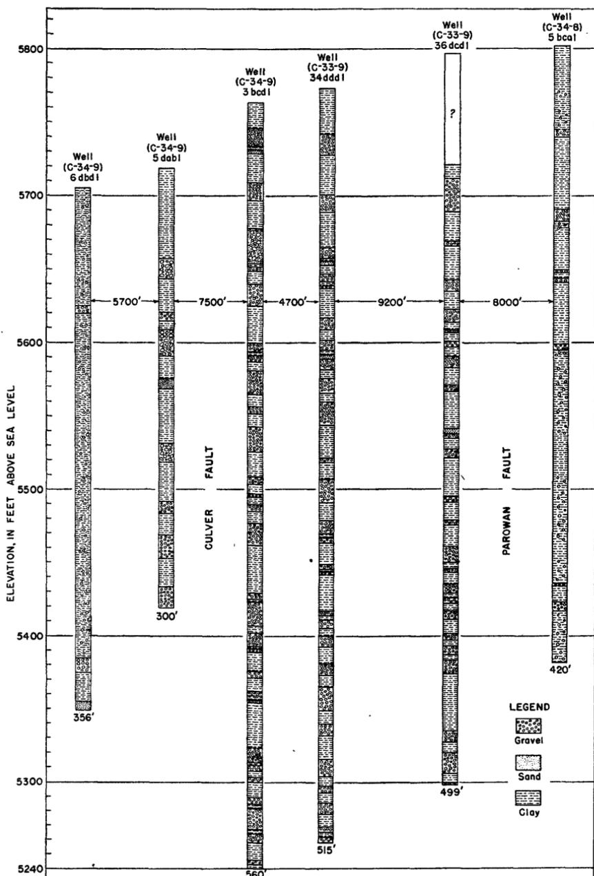
FIGURE 4.—Logs of six wells in Parowan Valley that are located near the east-west line that forms the south boundary of T. 33 S.
