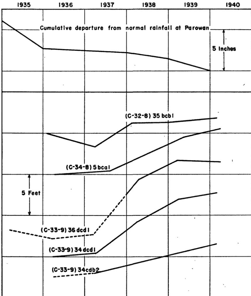
FIGURE 16.—Hydrographs showing annual high-water levels in five wells in Parowan Valley, 1935-40.
