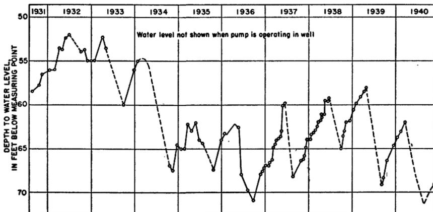
FIGURE 8.—Hydrograph of well (C-35-11) 33aac1, 1931-40.
